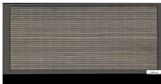
Fig. 1 Optical micrograph of TriA-X CFRP of 64 plies ( t = 8.8 mm)
