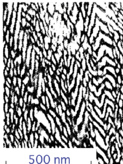
Fig. 2 Deformation of the lamellar microdomain structure by uniaxial stretching.
